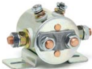
24401 SPDT Double-action Solenoid 85A at 12V DC. Use a pair of these solenoids in a reversing circuit. 12V 24401, 24V 24402, 36V 24400.
